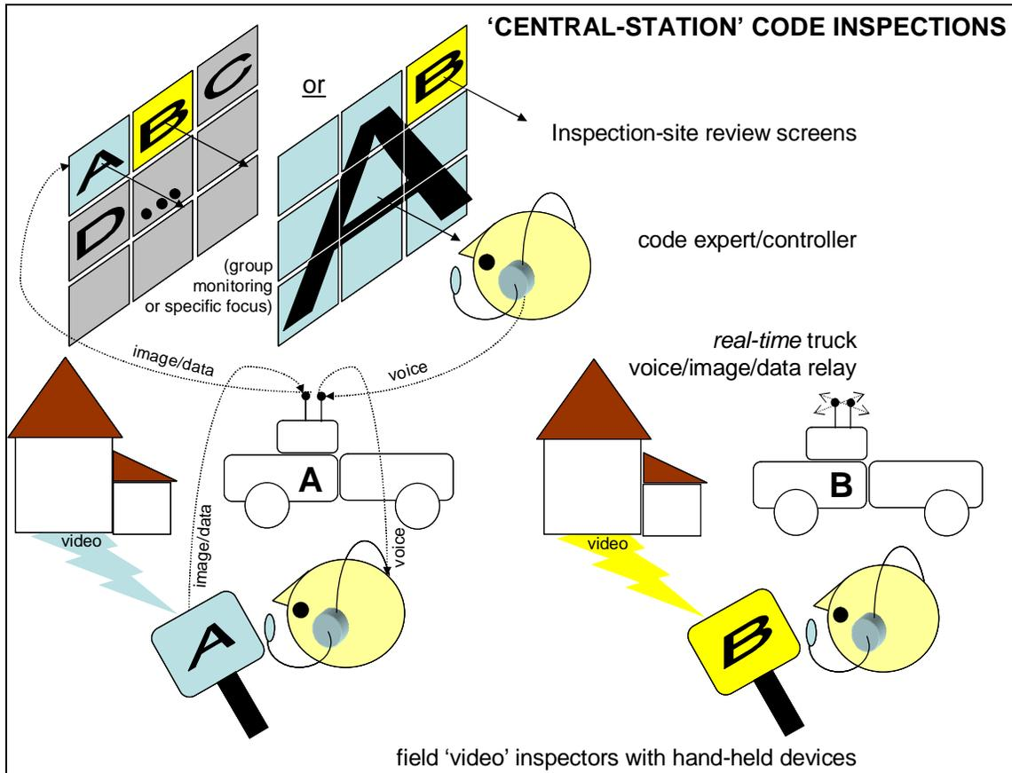
Figure 15 illustrates how we might put together all of the emerging technologies discussed in foregoing sections to create a “virtual” inspection in which a less-experienced person takes a (Level IV) handheld video device to a job site and then follows instructions from an expert code inspection team at a central site.
